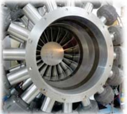
Experimental Fan Test Rig for Active Fan-Noise Control
