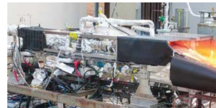
Precooled Turbojet Engine (Courtesy of JAXA)
